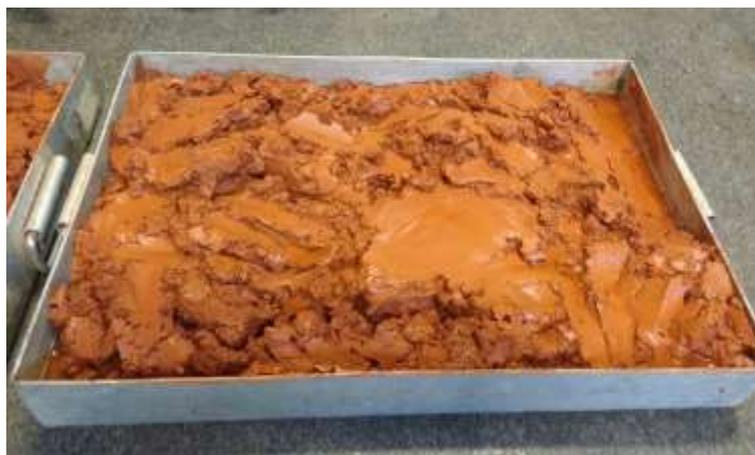
**FIGURA 16** - CONSISTÊNCIA PASTOSA DA LAMA VERMELHA. FONTE: AUTOR.
