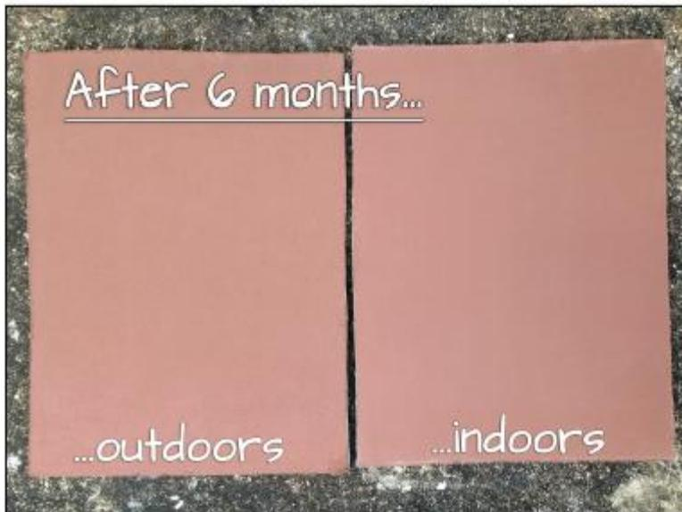
Results of the durability test after 6 months exposed to the external environment: rain, UV radiation and hail. These boards painted with PVA resin presented less than 3% variation on their colour and texture. This result was obtained through an image analysis software. Those painted with lime also showed low variability, around 5%. This result highlights the pigment potential of IOT. For comparison, conventional PVA paint decayed 12% after only 6 months of exposure, and the acrylic one, 3.4%.
