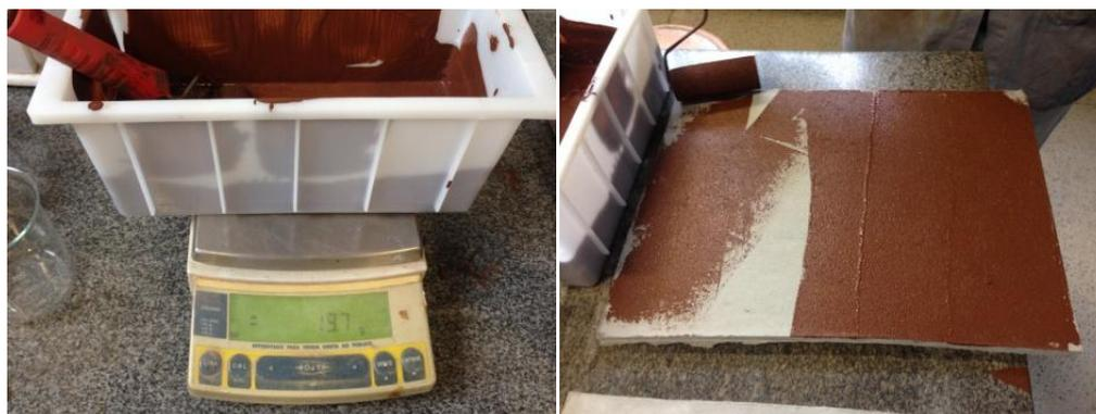
**Figura 26- PESAGEM INICIAL DA TINTA E PRIMEIRA DEMÃO NA PLACA CIMENTÍCIA**
