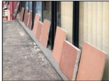
Durability test: boards exposed to sun, rain, hail and wind
