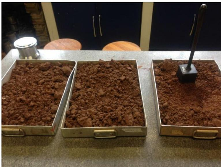
**Figura 6- RBMF APÓS 24 HORAS NA ESTUFA A 100°C**
