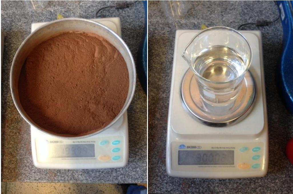
**Figura 11- PESAGEM DE RBMF E ÁGUA**
